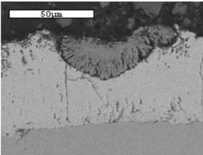
Figure 4. Non-bonded Corrosion Test. 2,000 hours ASTM B117 Salt Spray.
