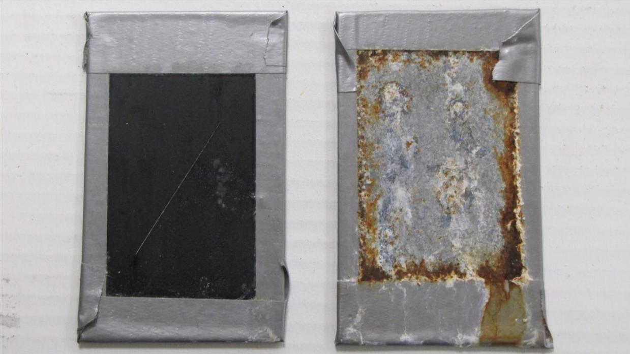
Figure 4b. Non-Bonded Panel after 2,000 hours of exposure. Thermal Diffusion Coating with waterborne top coat
