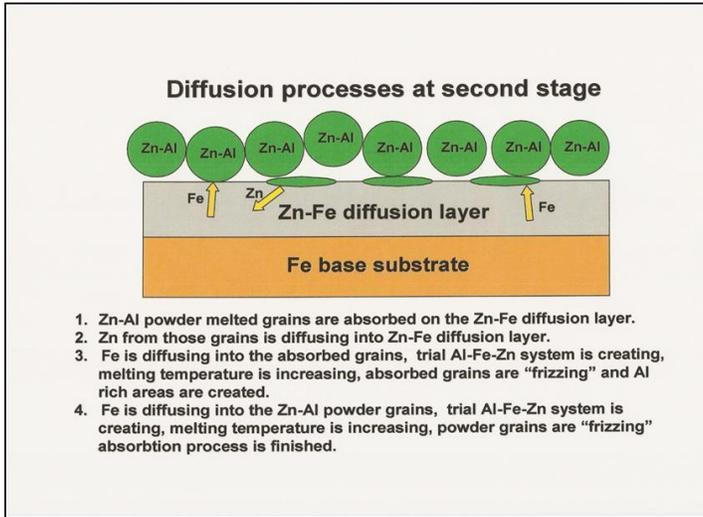
**Figure 2c. Thermal Diffusion Process – Final Coating Structure**
